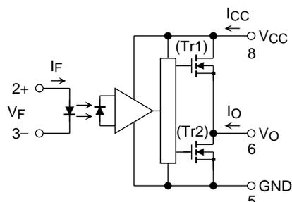
A 0.1  $\mu\text{F}$  bypass capacitor must be connected between pin 8 and 5.
