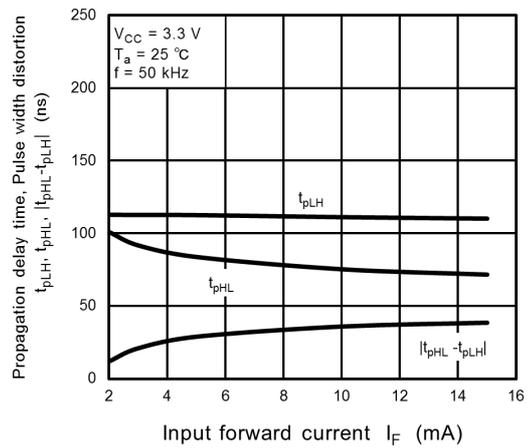
Fig. 12.2.18  $t_{pHL}, t_{pLH}, |t_{pHL} - t_{pLH}| - I_F$
