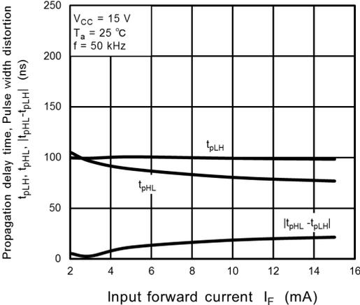
Fig. 12.2.19  $t_{pHL}, t_{pLH}, |t_{pHL} - t_{pLH}| - I_F$
