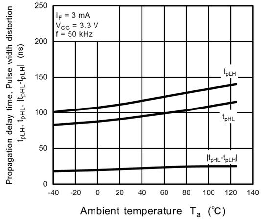
Fig. 12.2.14  $t_{pHL}, t_{pLH}, |t_{pHL} - t_{pLH}| - T_a$
