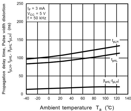
Fig. 12.2.15  $t_{pHL}, t_{pLH}, |t_{pHL} - t_{pLH}| - T_a$
