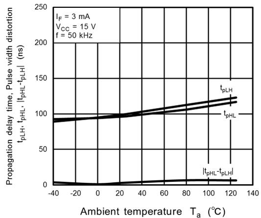
Fig. 12.2.16  $t_{pHL}, t_{pLH}, |t_{pHL} - t_{pLH}| - T_a$
