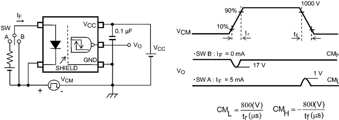
Fig. 12.1.8 Common-Mode Transient Immunity Test Circuit and Waveform
