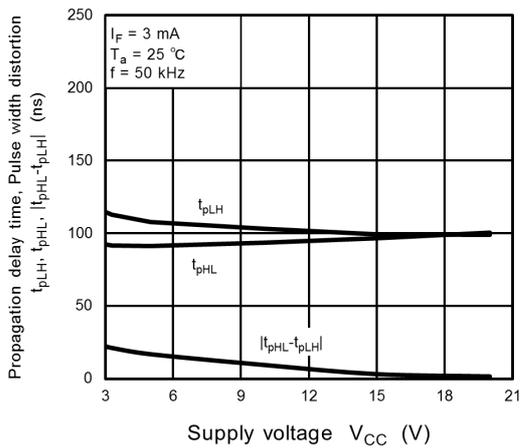
Fig. 12.2.17  $t_{pHL}, t_{pLH}, |t_{pHL} - t_{pLH}| - V_{CC}$
