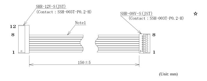
Note1: Cable: UL10368 (105°C 300V) AWG#30, diameter: φ0.8mm, Cable color: white. (Hitachi Cable Fine-Tech, Ltd.)
