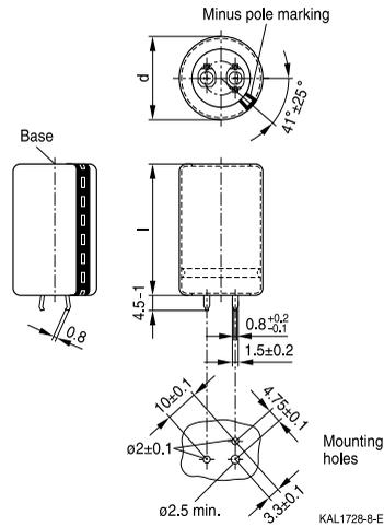
Large-size capacitors, snap-in terminals, length (6.3±1) mm. Also available in a shorter version with a length of (4.5–1) mm. Pressure relief device on the base.
