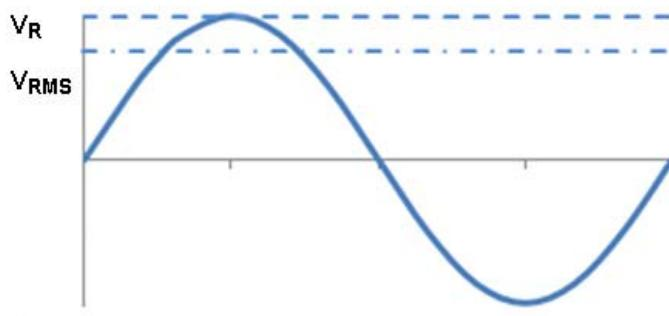
The root mean square of the maximum permissible value of the sinusoidal AC voltage in continuous operation.
