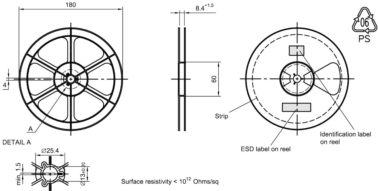
**Figure 19:** Drawing of reel (first-angle projection) with diameter of 180 mm.
