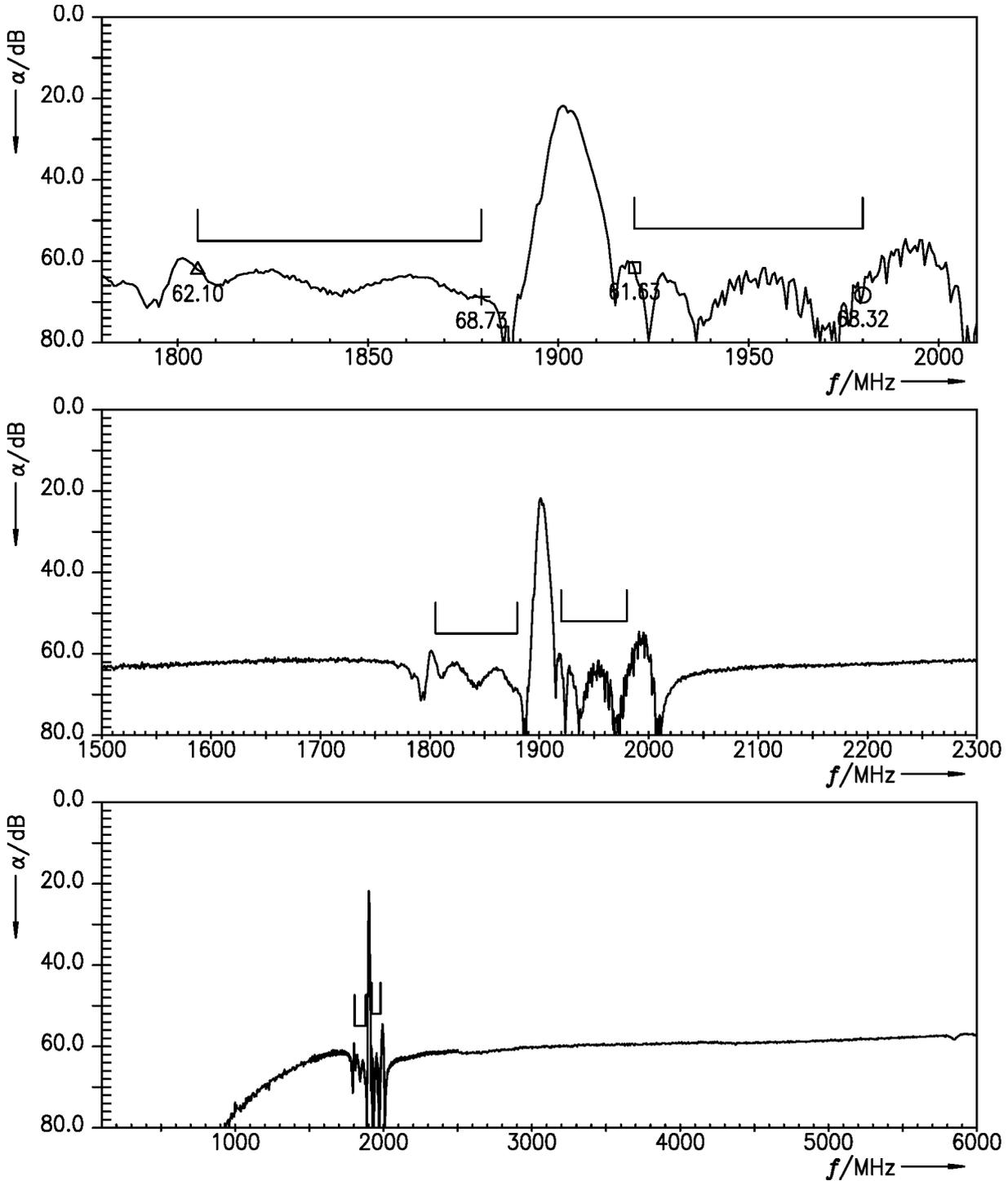
**Figure 16:** Cross-isolation LTE B1 TX – LTE B3 RX.
