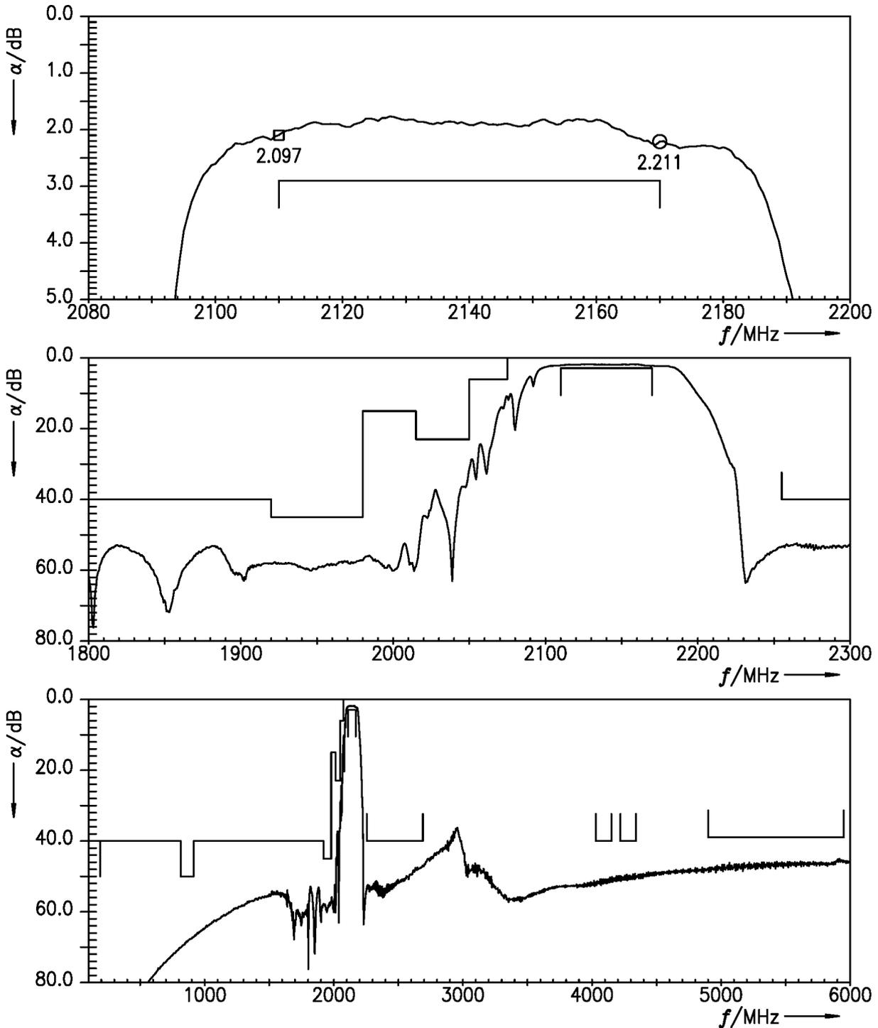
Figure 5: Attenuation LTE B1 ANT – RX.
