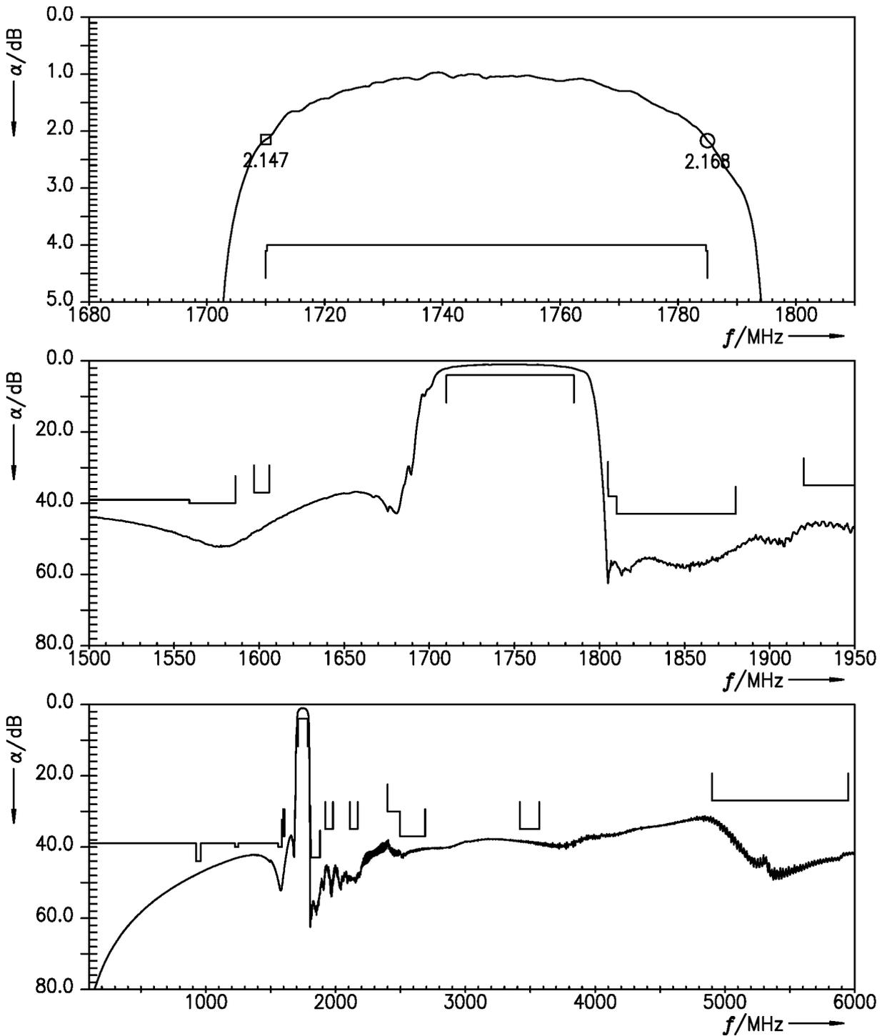
**Figure 10:** Attenuation LTE B3 TX – ANT.
