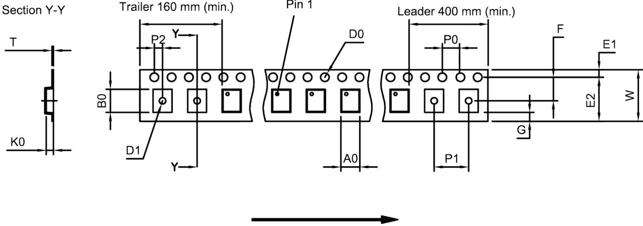
**Figure 18:** Drawing of tape (first-angle projection) with tape dimensions according to Table 1.
