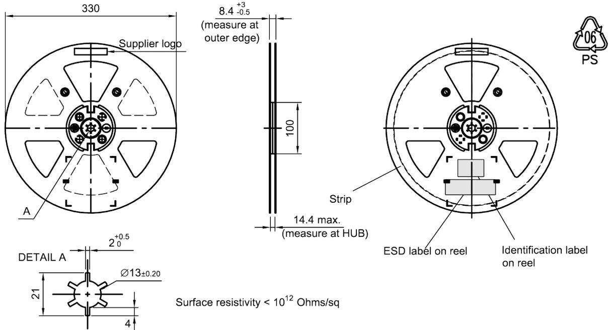
**Figure 22:** Drawing of reel (first-angle projection) with diameter of 330 mm.
