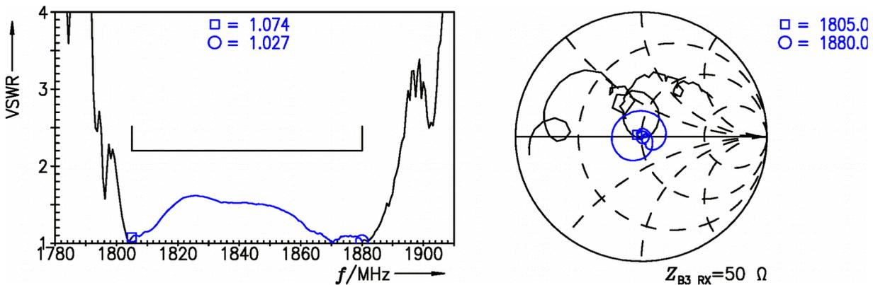
Figure 15: Reflection coefficient LTE B3 at RX port.
