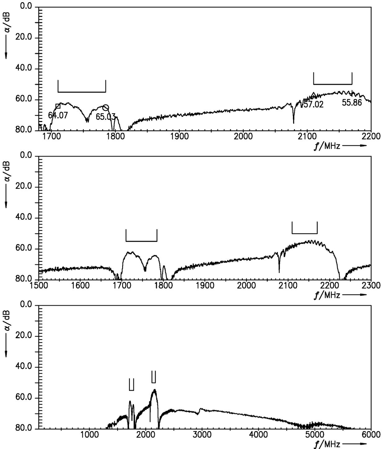
Figure 17: Cross-isolation LTE B3 TX – LTE B1 RX.
