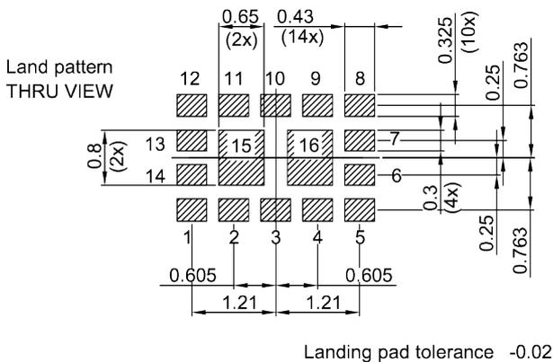
**Figure 2: Drawing of package with package height A = 0.5 mm (max.). See Sec. Package information (p. 32).**
