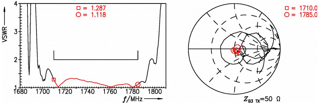
Figure 13: Reflection coefficient LTE B3 at TX port.
