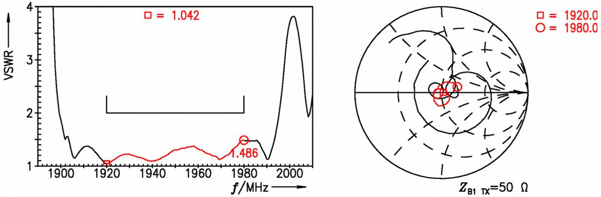
Figure 7: Reflection coefficient LTE B1 at TX port.
