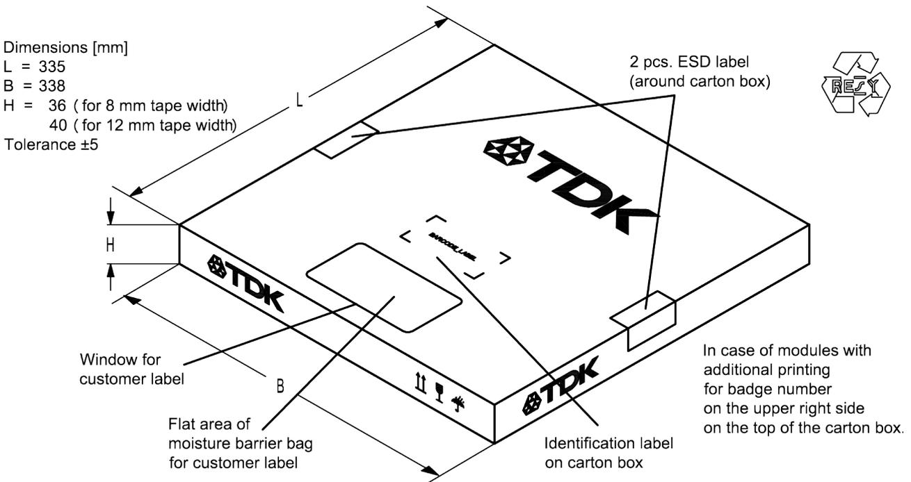
Figure 24: Drawing of folding box for reel with diameter of 330 mm.
