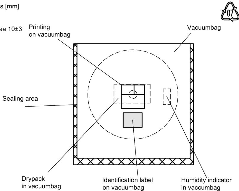
**Figure 23:** Drawing of moisture barrier bag (MBB) for reel with diameter of 330 mm.
