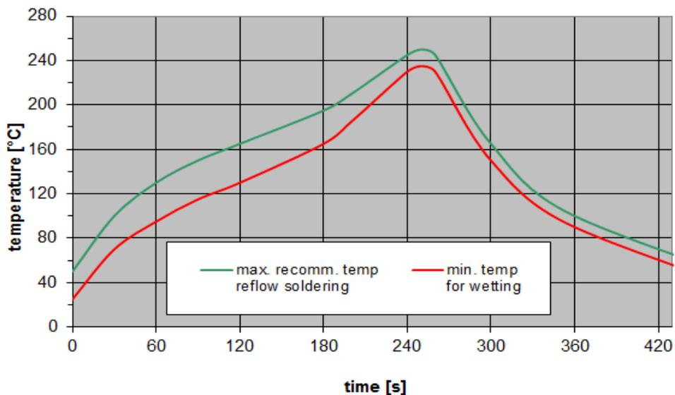
**Figure 25:** Recommended reflow profile for convection and infrared soldering – lead-free solder.
