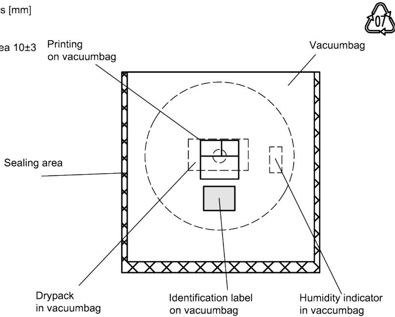
**Figure 20:** Drawing of moisture barrier bag (MBB) for reel with diameter of 180 mm.
