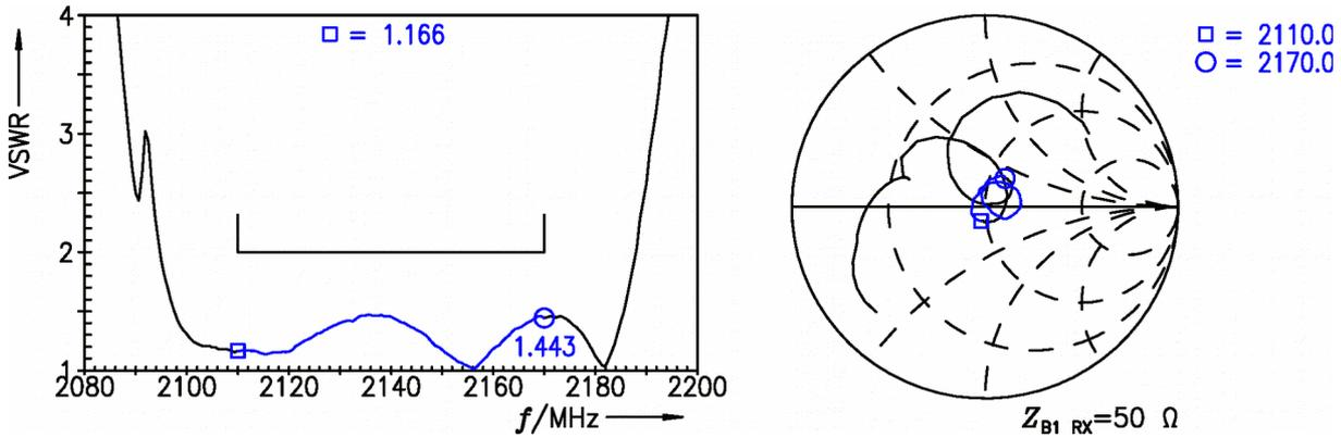
Figure 9: Reflection coefficient LTE B1 at RX port.
