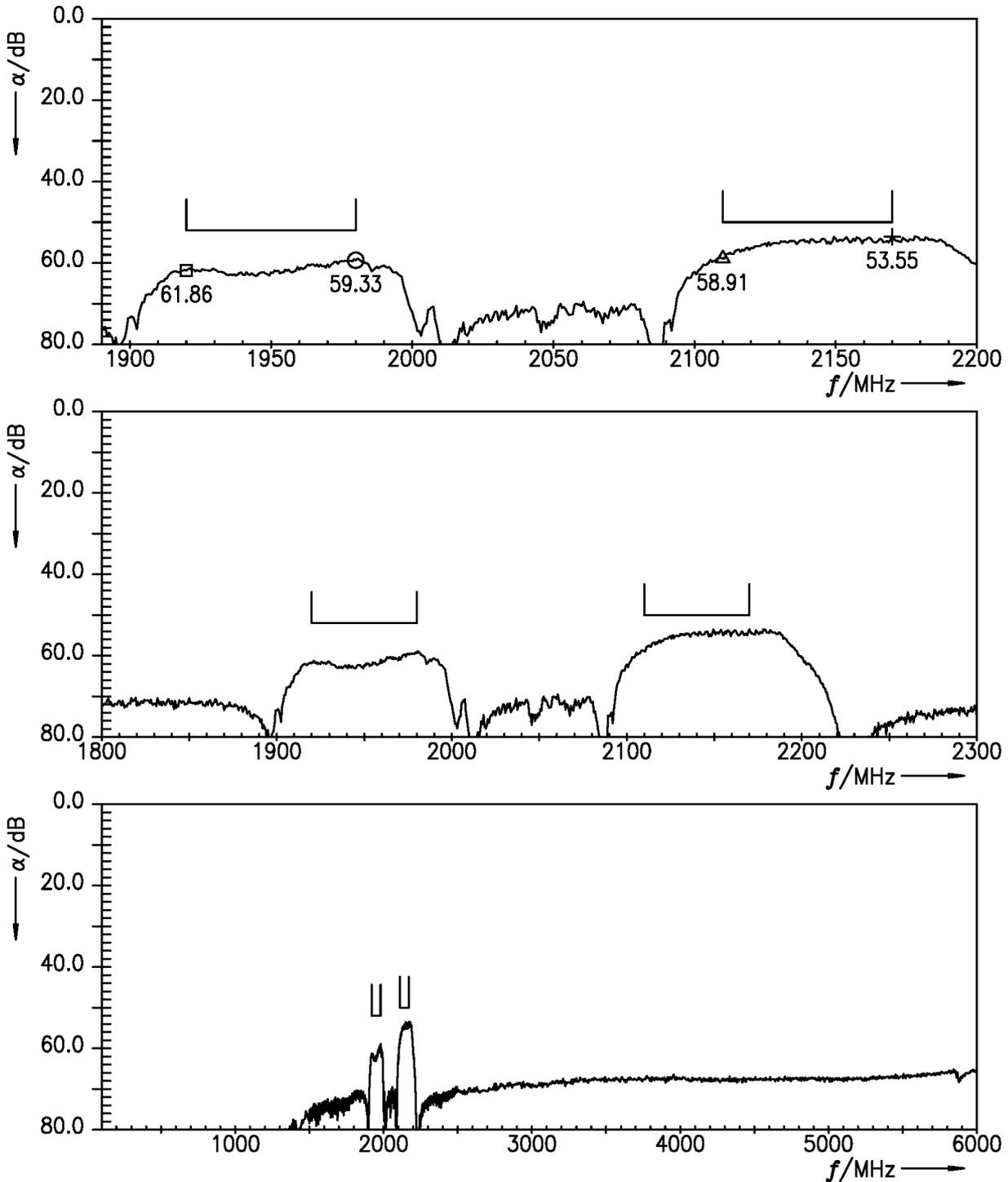
**Figure 6:** Isolation LTE B1 TX – RX.
