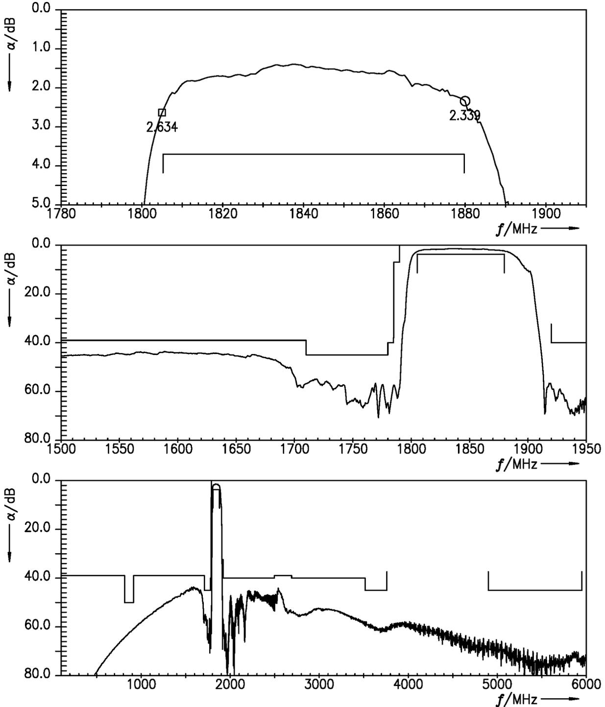
Figure 11: Attenuation LTE B3 ANT – RX.
