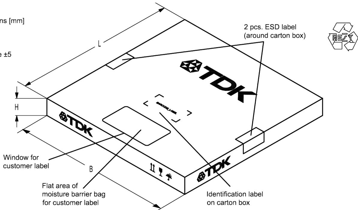
**Figure 21:** Drawing of folding box for reel with diameter of 180 mm.
