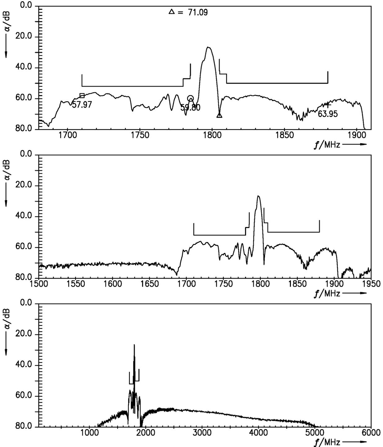
Figure 12: Isolation LTE B3 TX – RX.
