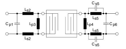
$C_{p1} = 4.7 \text{ pF}$   $L_{s2} = 3.6 \text{ nH}$   $L_{p3} = 39.0 \text{ nH}$   $L_{p4} = 91.0 \text{ nH}$   $L_{s5} = 11.0 \text{ nH}$   $C_{s5} = 18.0 \text{ pF}$  $C_{p6} = 1.0 \text{ pF}$
