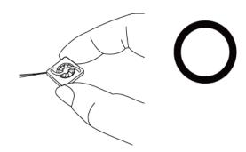
Don't pull fan with lead wires.
