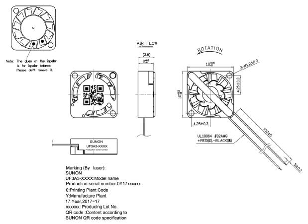
Sunon standard sample exclude the connector. If there is any request for connector, please advise in advance. About recommend connector, SUNON recommend the following models for SUNON Mighty Mini Fon/Blower: 1.(JST) SUR series connector: 02SUR-32S / 03SUR-32S / 04SUR-32S.
