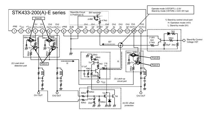
The protection circuit application for the STK433-200(A)-Esr consists of the following blocks (blocks (1) to (4)).
