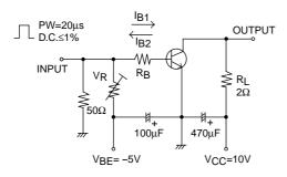
$I_{C}=10I_{B1}=-10I_{B2}=5A$  (For PNP, the polarity is reversed.)
