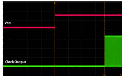
Figure 17. Startup Waveform vs. Vdd
