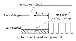
Figure 4. Startup Timing (OE/ST Mode)
