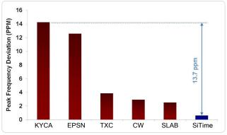
Figure 6. Shock Robustness<sup>[6]</sup>
