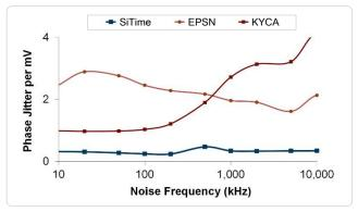
Figure 4. Power Supply Noise Rejection<sup>[4]</sup>
