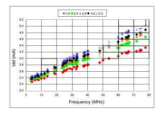
Figure 8. Idd vs Frequency
