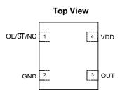
Figure 1. Pin Assignments
