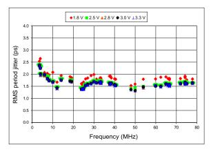
Figure 10. RMS Period Jitter vs Frequency
