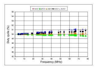
Figure 11. Duty Cycle vs Frequency
