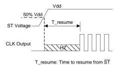
Figure 5. Standby Resume Timing (ST ModeOnly)
