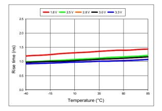
Figure 12. 20%-80% Rise Time vs Temperature
