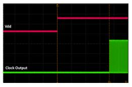
Figure 17. Startup Waveform vs. Vdd
