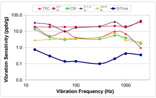
Figure 5. Vibration Robustness<sup>[5]</sup>
