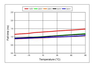
Figure 13. 20%-80% Fall Time vs Temperature
