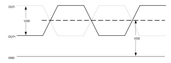
Figure 6. LVDS Voltage Levels per Differential Pin (i.e. OUT+, or OUT-)
