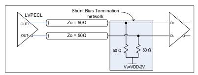
Figure 13. LVPECL and Low-swing LVPECL with DC-coupled Parallel Shunt Load Termination
