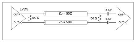
Figure 15. LVDS double AC Termination with Capacitor Close to the Load
