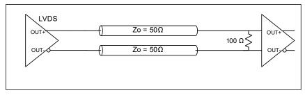
Figure 14. LVDS Single DC Termination at the Load
