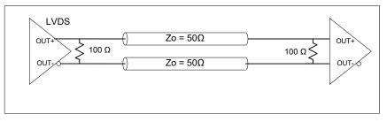
Figure 16. LVDS Double DC Termination
