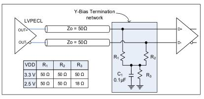
Figure 12. LVPECL and Low-swing LVPECL with Y-Bias Termination
