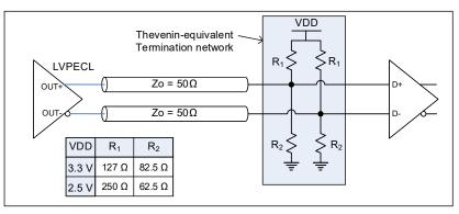
Figure 11. LVPECL and Low-swing LVPECL DC-coupled Load Termination with Thevenin Equivalent Network
