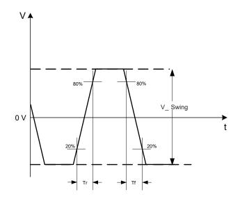
Figure 5. LVPECL, Low-swing LVPECL, and HCSL Voltage Levels Across Differential Pair (i.e. OUT+ minus OUT-)
