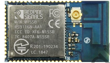
LGA Module (AA1) 27 mm x 16 mm
