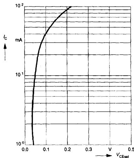
**Input off voltage  $V_{i(off)} = f(I_C)$**
