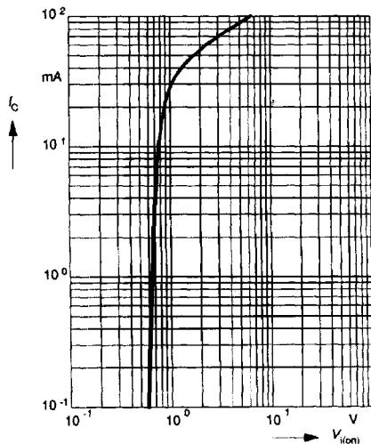
**Collector-Emitter Saturation Voltage**
