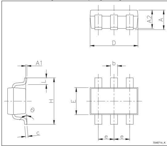
Figure 19. SOT23-6L package drawing
