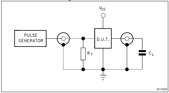
1.  $C_L$  = 50 pF or equivalent (includes jig and probe capacitance)  $R_T$  =  $Z_{OUT}$  of pulse generator (typically 50  $\Omega$ ).
