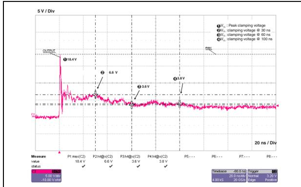
Figure 7. ESD response to IEC 61000-4-2 (-15 kV contact discharge)
