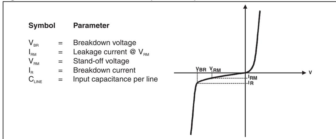
**Table 2. Electrical characteristics (values,  $T_{amb} = 25\text{ }^\circ\text{C}$ )**
