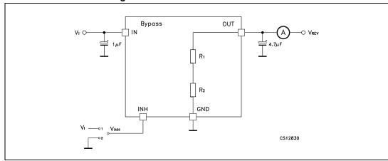
Figure 22. Reverse current test circuit
