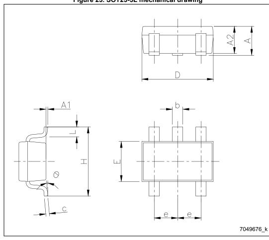
Figure 23. SOT23-5L mechanical drawing
