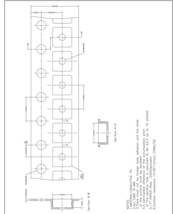
Figure 25. SOT23-5L reel mechanical drawing
