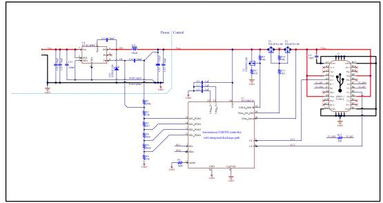
The STUSB4710 offers the possibility to have up to 5 PDOs using (GPIO0 to GPIO3).
