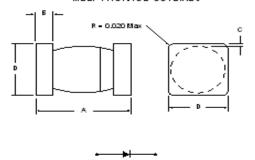
Note: Cathode side of device is indicated by a dark band marked on body.
