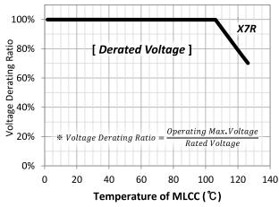
This product ,which guarantees High Temperature Reliability Test with 100% of rated voltage at the maximum temperature, is recommended to be used in the circuit with derated voltage compared to the rated voltage of the capacitor for long lifetime.
