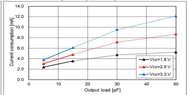
\* Output load condition under  $L_{CMOS} > 15\text{ pF}$  (dotted line area) is not guaranteed, and the data is for reference.
