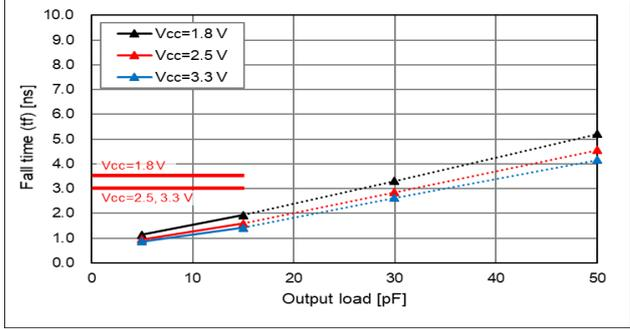
10% - 90% V<sub>CC</sub>, L<sub>CMOS</sub> = 15 pF, Temp. Char.
