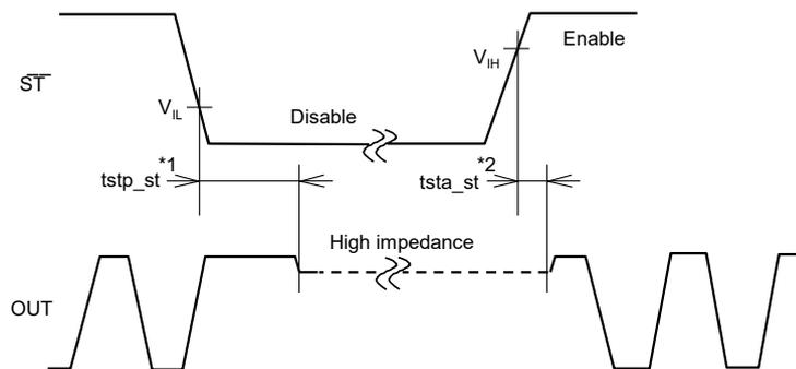
\*1 The period from  $\overline{ST} = V_{IL}$  to  $OUT = High\ impedance\ (Disable)$
