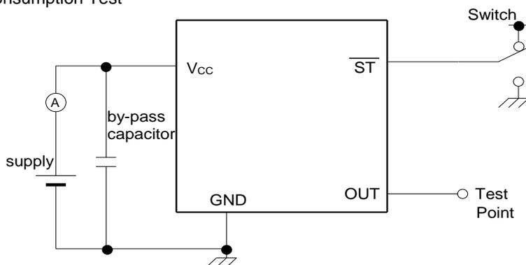
\*Standby current test should be  $\overline{ST} = \text{GND}$ .
