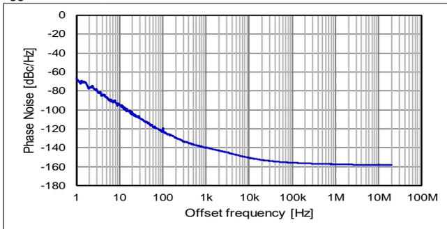
Phase Jitter (Offset frequency: 12 kHz to 20 MHz)
