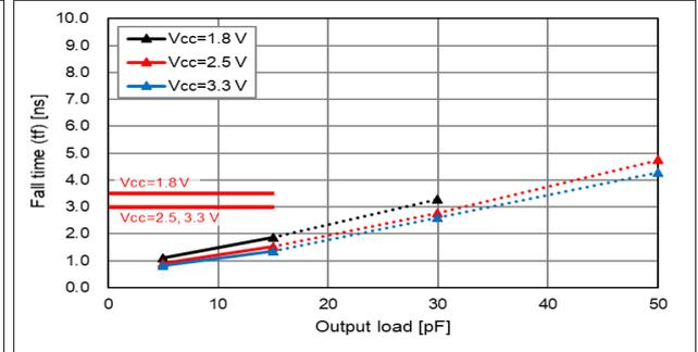
10% - 90% V<sub>CC</sub>, L<sub>CMOS</sub> = 15 pF, Temp. Char.
