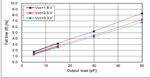
\* Output load condition under L<sub>CMOS</sub> > 15 pF (dotted line area) is not guaranteed, and the data is for reference.
