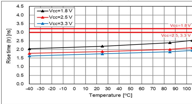
20% - 80% V<sub>CC</sub>, T<sub>use</sub> = +25 °C, Output load Char.
