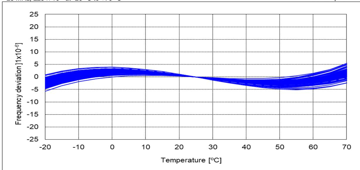
$f_0 = 25 \text{ MHz}$ ,  $\pm 50 \times 10^{-6}$  at  $-40 \text{ }^\circ\text{C}$  to  $+85 \text{ }^\circ\text{C}/+105 \text{ }^\circ\text{C}$
