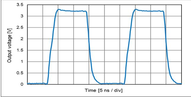
V<sub>CC</sub> = 2.5 V, L<sub>CMOS</sub> = 15 pF, T<sub>use</sub> = +25 °C
