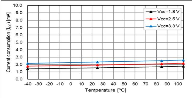
$T_{use} = +25\text{ }^{\circ}\text{C}$ , Output load( $L_{CMOS}$ ) Characteristics
