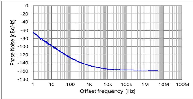
Phase Jitter (Offset frequency: 12 kHz to 5 MHz)
