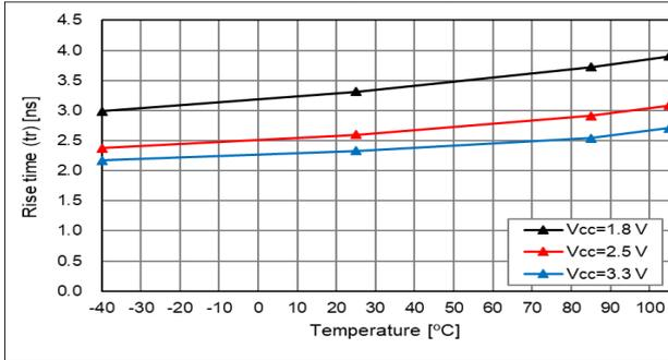
10% - 90% V<sub>CC</sub>, T<sub>use</sub> = +25 °C, Output load Char.
