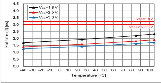
20% - 80% V<sub>CC</sub>, T<sub>use</sub> = +25 °C, Output load Char.
