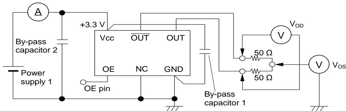
\* The lines from OUT and  $\overline{\text{OUT}}$  pin are same length.
