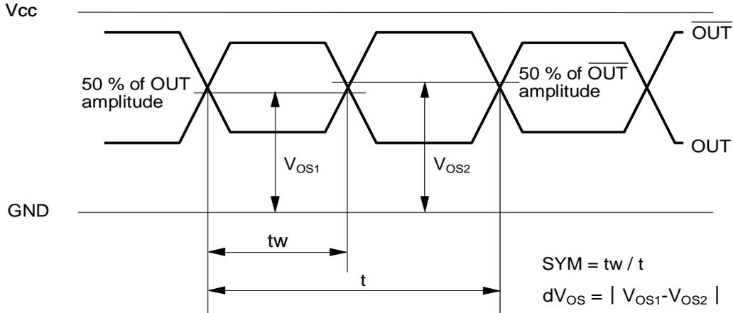
Differential output waveform (OUT -  $\overline{\text{OUT}}$ )
