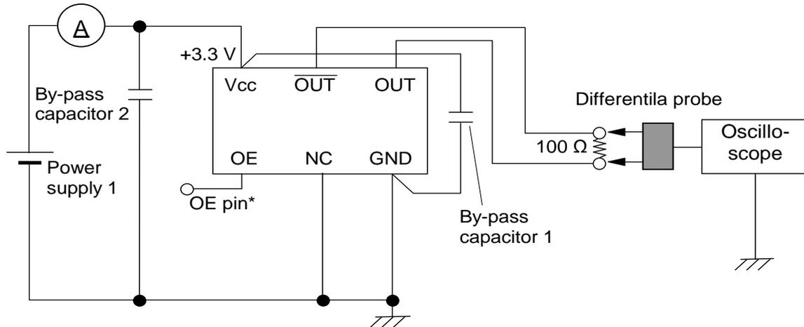
\* The lines from OUT and  $\overline{\text{OUT}}$  pin are same length.
