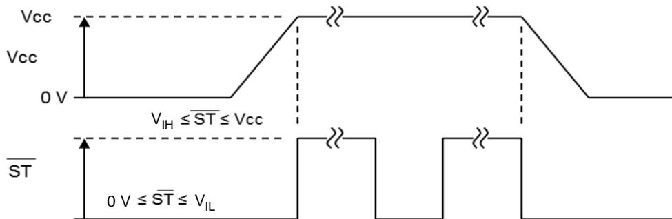
When standby control and  $V_{CC}$  control are the same
