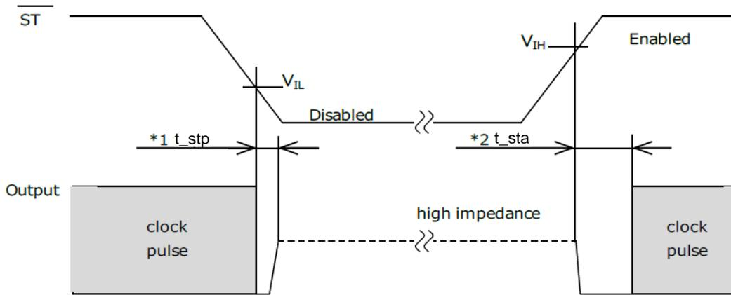
\*1  $t_{stp\_st}$ : The time from  $\overline{ST} = V_{IL}$  to output = disable (high impedance)
