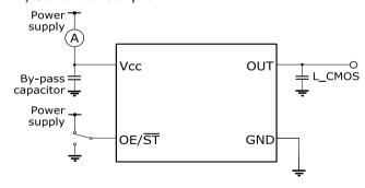
\* Current consumption under the disable function should be OE = GND Current consumption under the standby function should be ST = GND.
