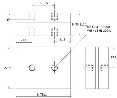
Tightening torque 15Nm max.
