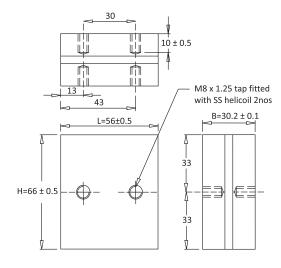
Tightening torque 15Nm max.
