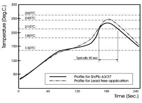
Infrared soldering profile for Chip Resistors
