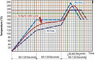
Infrared Soldering Profile
