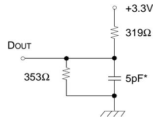
\* Capacitive Load consists of all components of the test environment.
