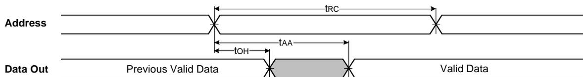
TIMING WAVEFORM OF READ CYCLE(2) ( $\overline{WE}=V_{IH}$ )
