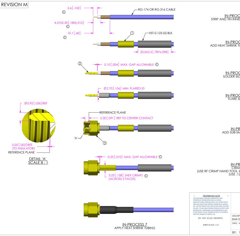
IN-PROCESS 1 STRIP AND TIN INNER CONDUCTOR
