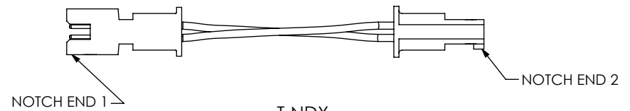
T-NDX (END 2 NOTCH DOWN, CABLE CROSSED) (PIN 1 TO PIN 2)
