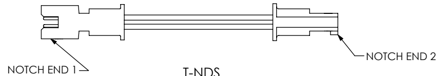
T-NDS (END 2 NOTCH DOWN, CABLE STRAIGHT) (PIN 1 TO PIN 1)
