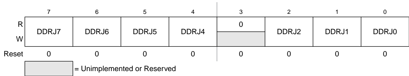
Figure 22-58. Port J Data Direction Register (DDRJ)
