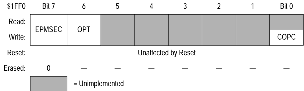
Figure 13-3. EPROM Security in COP Register (COP)
