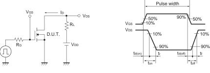
Fig.1-1 Switching time measurement circuit
