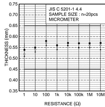
Fig.4 Dimensions (thickness)
