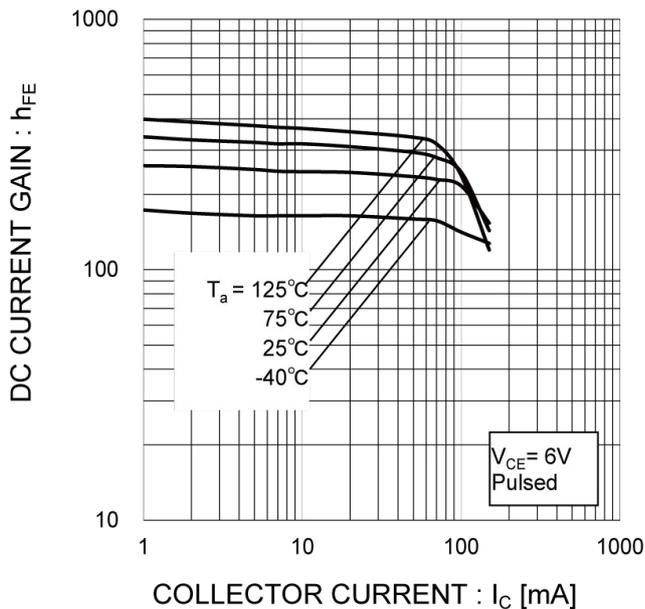
Fig.16 DC Current Gain vs. Collector Current (II)
