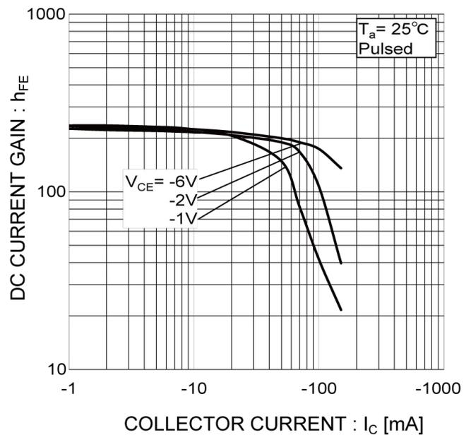
●Electrical characteristic curves( $T_a=25^\circ\text{C}$  <For Tr1(PNP)>
