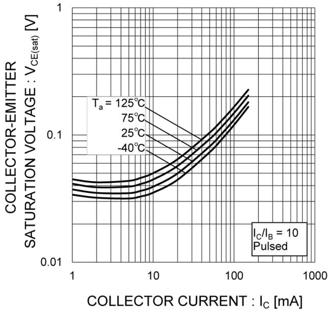
Fig.18 Collector-Emitter Saturation Voltage vs. Collector Current(II)
