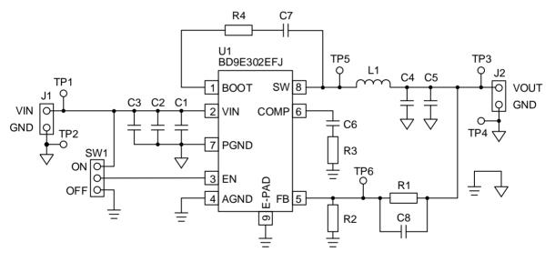
Figure 3. BD9E302EFJ-EVK-001 Circuit Diagram
