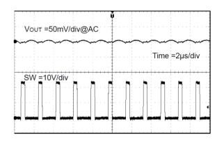
Figure 14. Output Voltage Ripple Wave  $(V_{\text{IN}}{=}24\text{V})$
