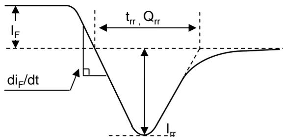
Fig.24 Diode Reverse Recovery Waveform
