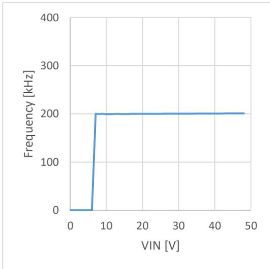
Figure 12. Switching Frequency vs VIN
