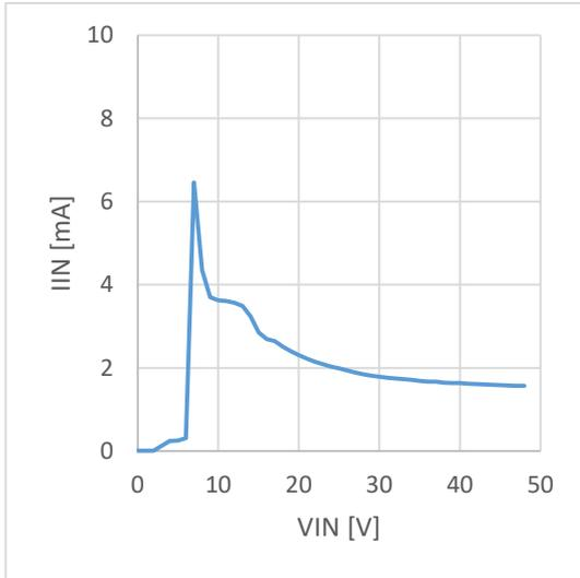
Figure 8. Current Consumption vs VIN
