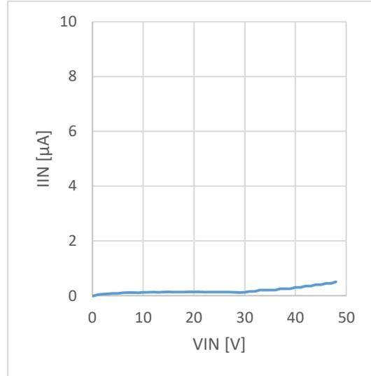
Figure 9. Shutdown Current vs VIN
