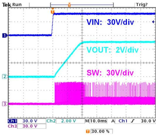
Figure 16. Start Up Waveform
