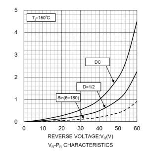
REVERSE POWER DISSIPATION:P<sub>R</sub>(W)
