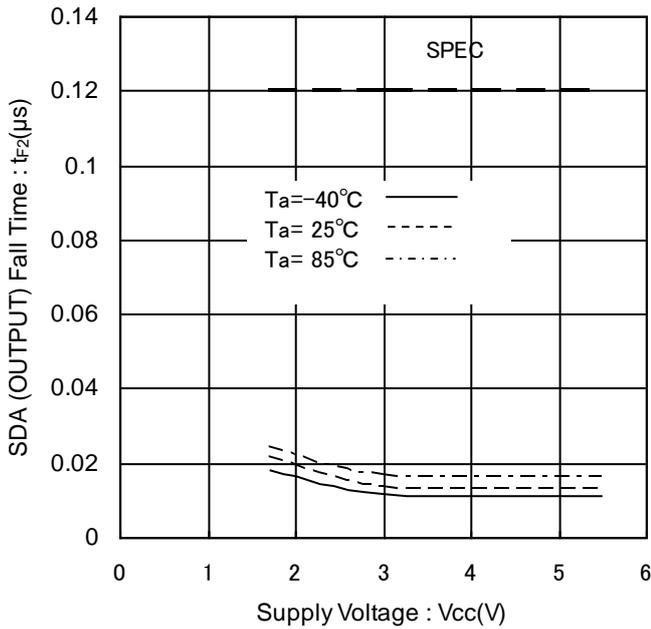
Figure 16. SDA (OUTPUT) Fall Time vs Supply Voltage
