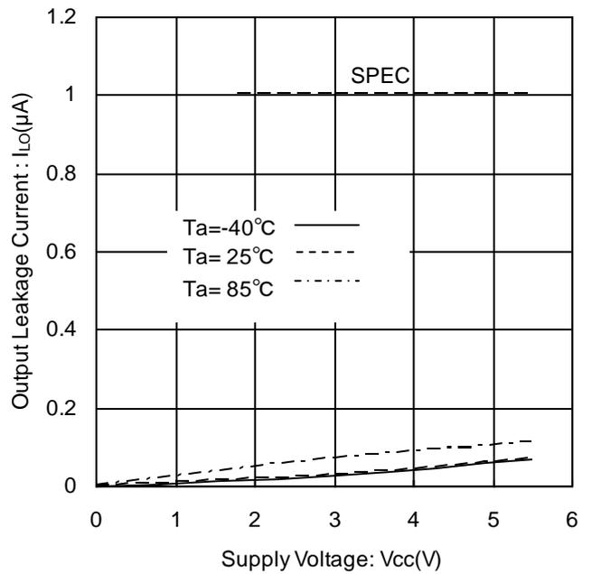
Figure 9. Output Leakage Current vs Supply Voltage (SDA)
