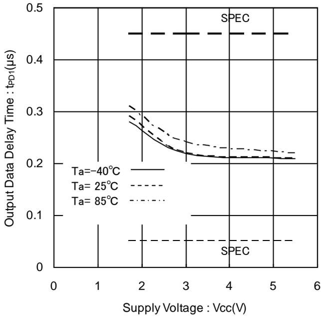
Figure 24. Output Data Delay Time vs Supply Voltage
