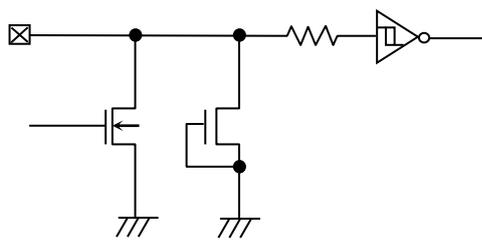
Figure 51. Input / Output Pin Circuit Diagram
