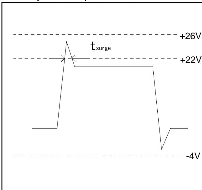
**●Waveform for switching test**
