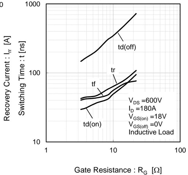
Fig.19 Switching Characteristics vs. Gate Resistance [  $T_j=125^{\circ}\text{C}$  ]
