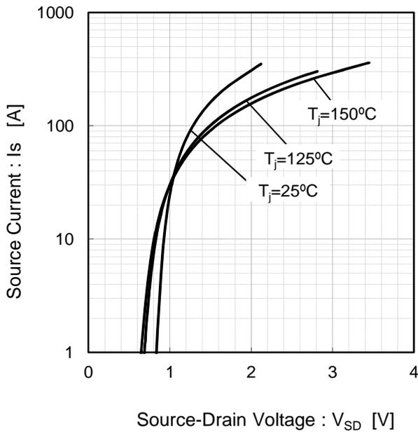
Fig.6 Forward characteristic of Diode
