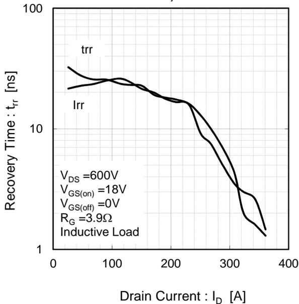
Fig.16 Recovery Characteristics vs. Drain Current [  $T_j=125^{\circ}\text{C}$  ]
