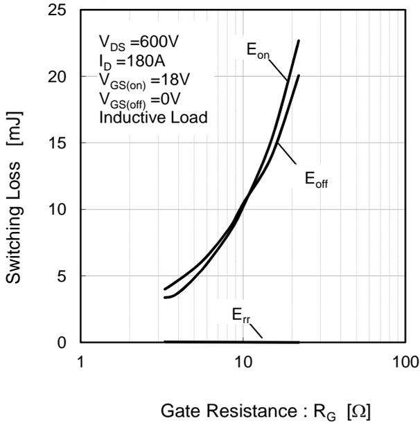
Fig.22 Switching Loss vs. Gate Resistance [  $T_j=125^{\circ}\text{C}$  ]
