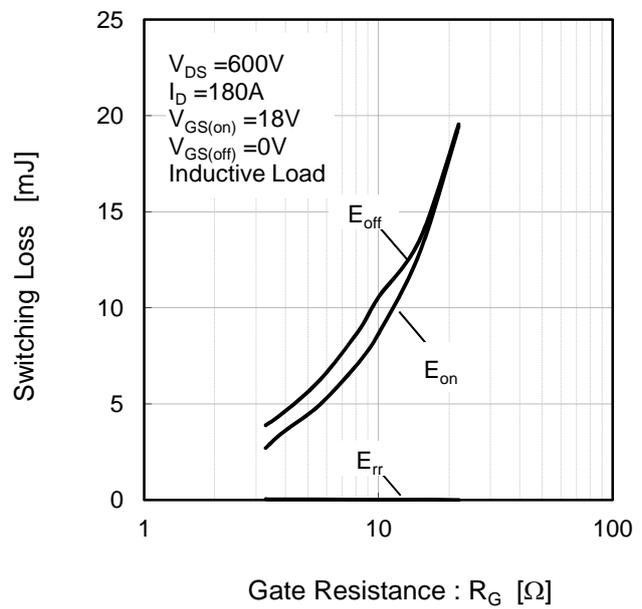
Fig.23 Switching Loss vs. Gate Resistance [  $T_j=150^{\circ}\text{C}$  ]
