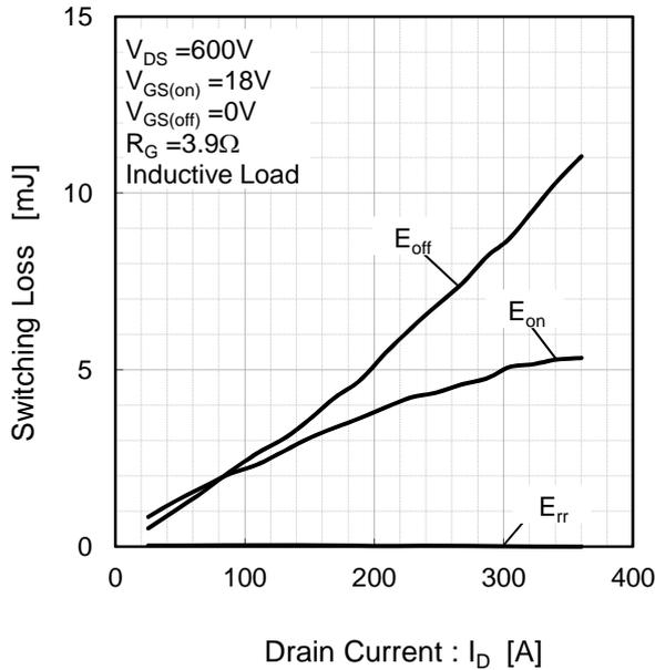
Fig.14 Switching Loss vs. Drain Current [  $T_j=150^{\circ}\text{C}$  ]
