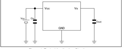
Figure 1. Typical Application Circuit
