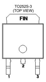
Figure 2. Pin Configuration
