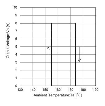
Figure 12. Thermal Shutdown Circuit Characteristic
