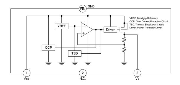
Figure 3. Block Diagram
