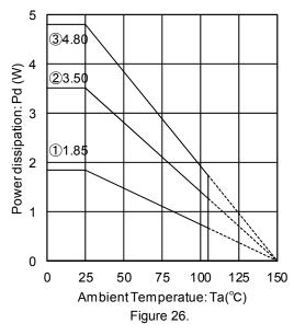
IC mounted on a ROHM standard board Board size : 70mm×70mm×1.6mm Copper area : 7mm×7mm
