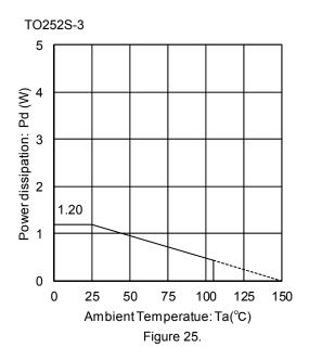
Mounted on a Rohm standard board Board size : 70mm × 70 mm × 1.6 mm Copper foil area :7mm × 7mm
