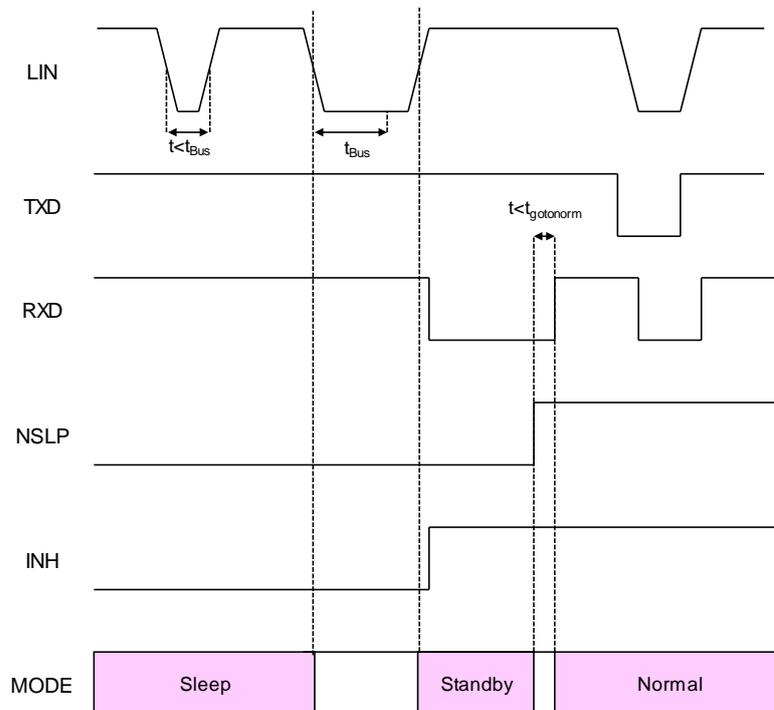
Figure 7. Remote wake-up (Sleep→Standby→Normal)
