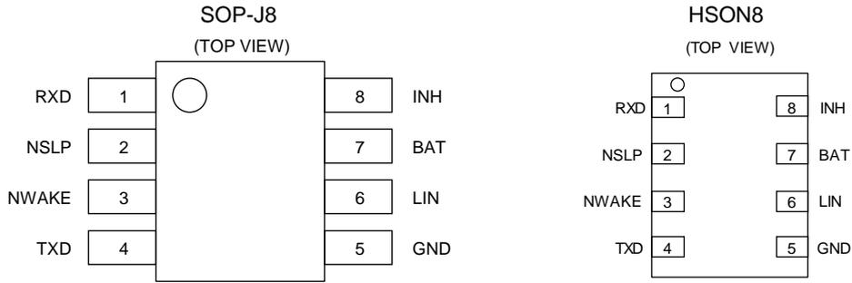
Figure 2. Pin Configuration
