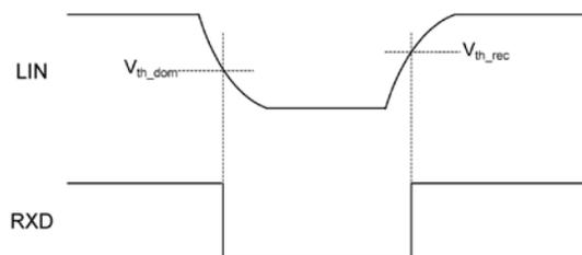
(Note 4) Load condition at bus ( C<sub>L(LIN-GND)</sub>; R<sub>L(LIN-BAT)</sub> ) : 1nF;1kΩ / 6.8nF;660Ω / 10nF;500Ω
