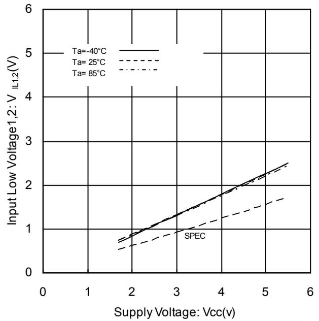
Figure 5. Input Low Voltage1,2 vs Supply Voltage
