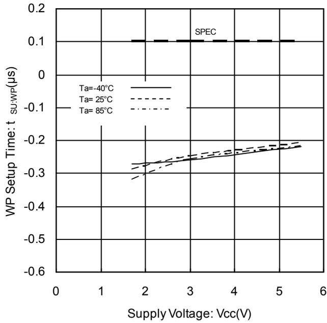
Figure 32. WP Setup Time vs Supply Voltage
