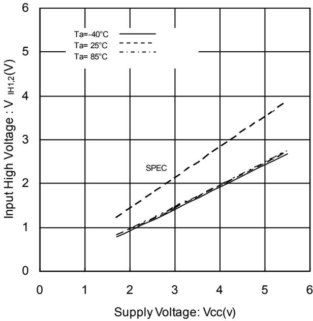
Figure 4. Input High Voltage1,2, vs Supply Voltage
