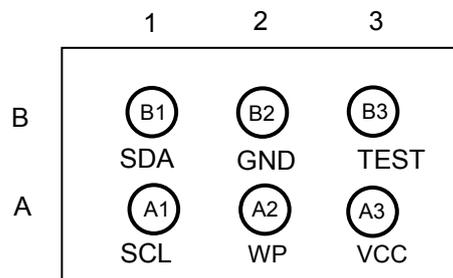
Figure 3. Pin Configuration
