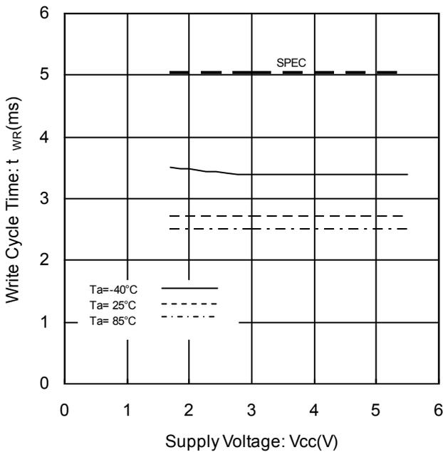
Figure 26. Write Cycle Time vs Supply Voltage
