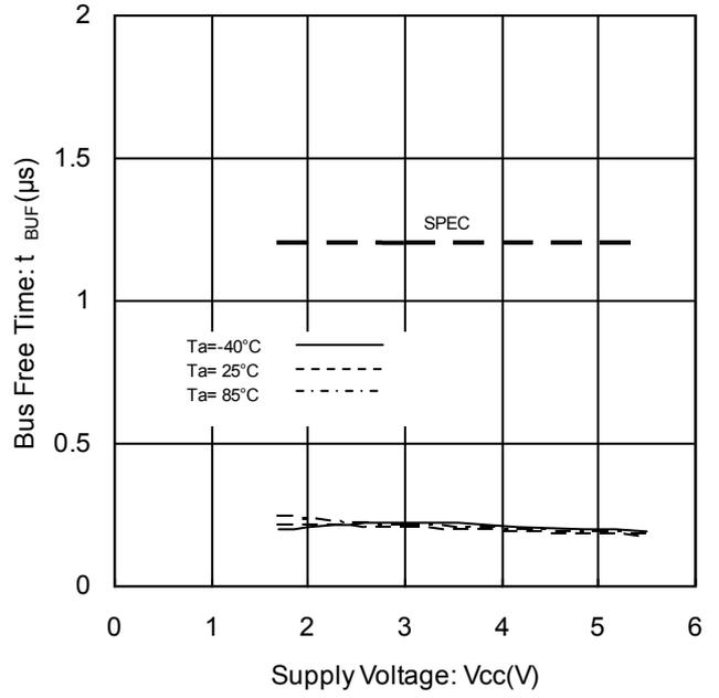
Figure 25. Bus Free Time vs Supply Voltage
