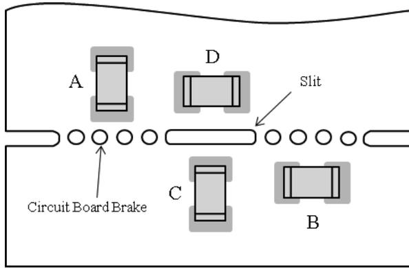
Stress strength according to the mounting position:
