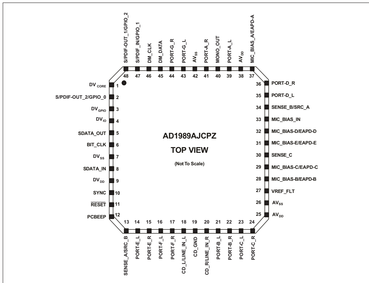
Figure 1. AD1989A Pinout
